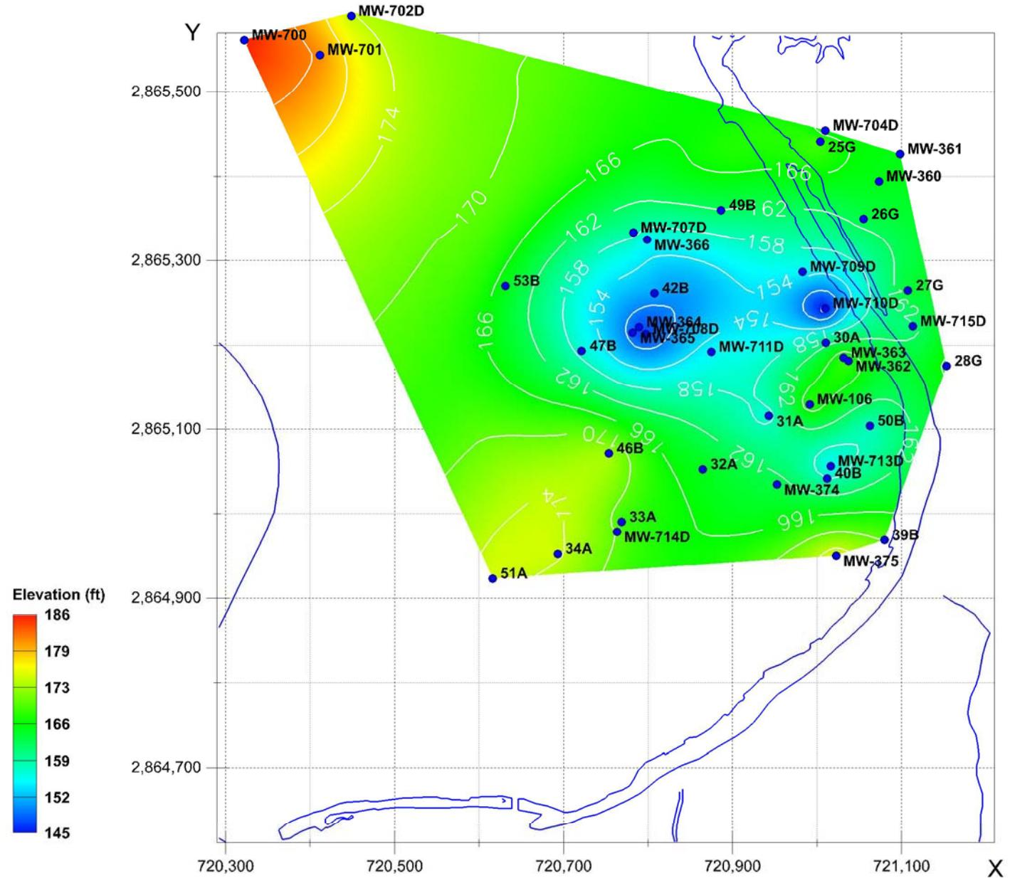
Figure 11 – Bedrock Elevations from Drilling
