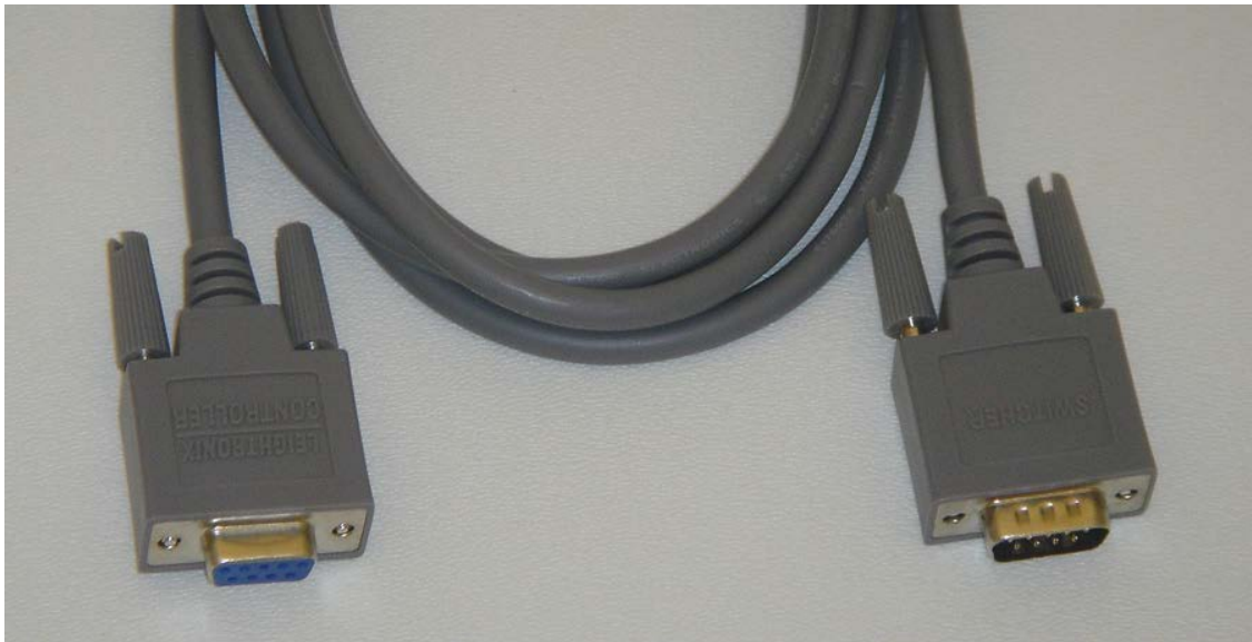
Illustration 291, DB9F-DB9M Straight-Through Cable, Part #10-4869
