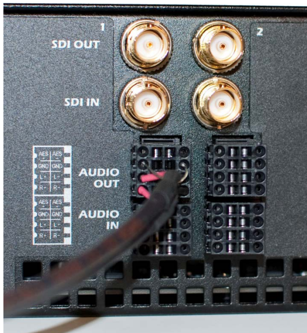
Illustration 27, Example of Audio Terminal Block Wired for Analog and Connected to Rear Panel
