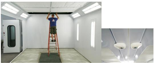
Full down draft airflow (raised basement) spray & curing cycles / full filtered ceiling plenum.
