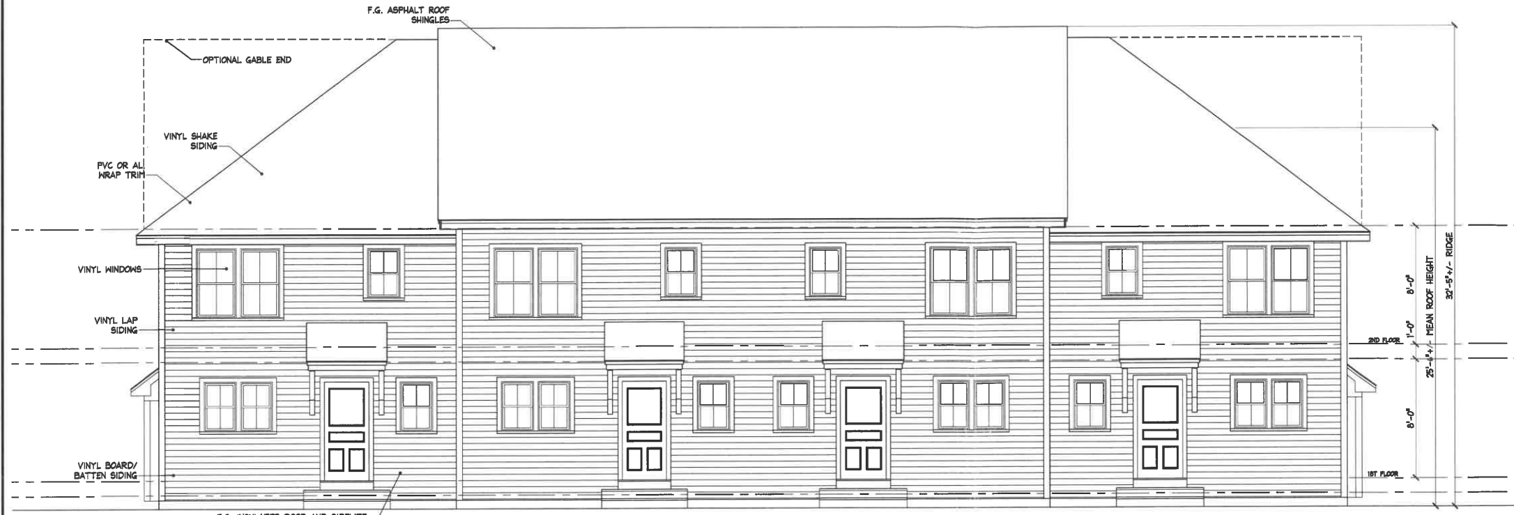
TYPICAL 4 UNIT BUILDING REAR ELEVATION 1/4" = 1'-0"
