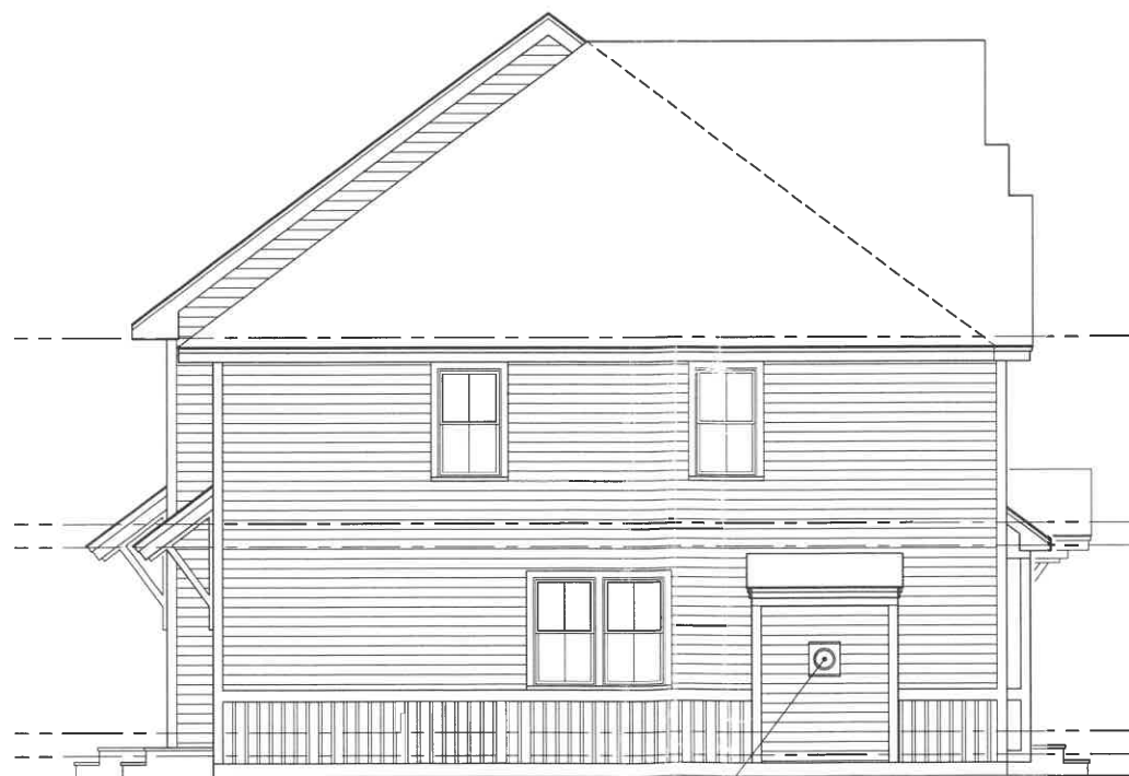
TYPICAL 4 UNIT BUILDING LEFT ELEVATION 1/4" = 1'-0"
