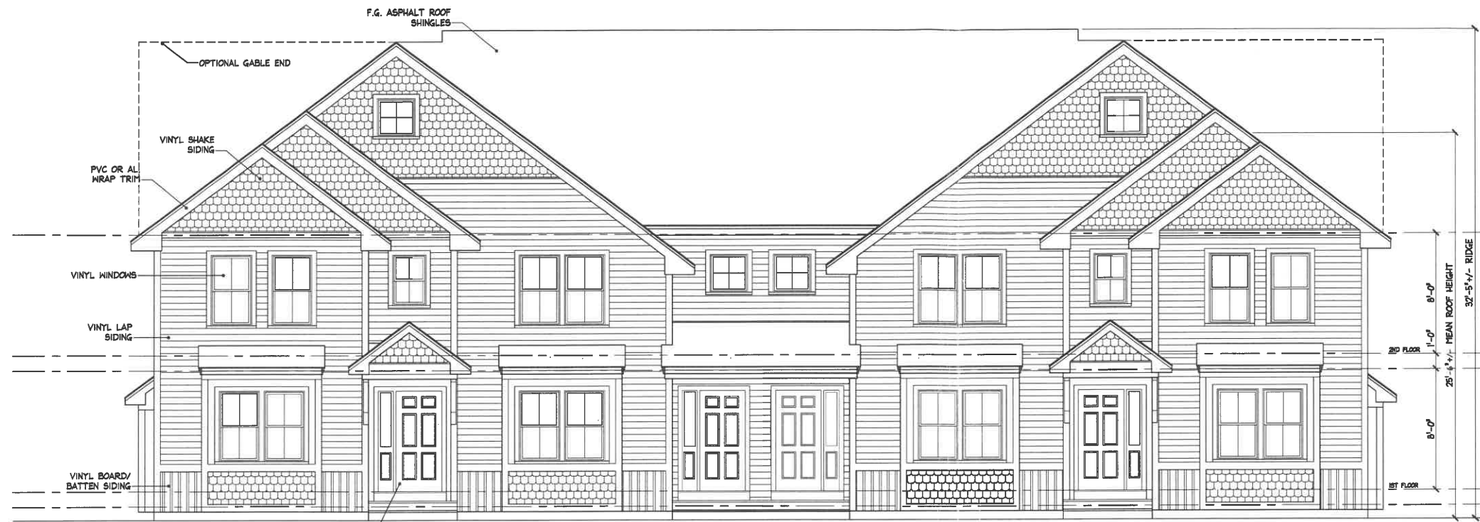
TYPICAL 4 UNIT BUILDING FRONT ELEVATION 1/4" = 1'-0"
