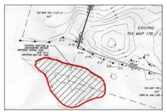
A certified pool is located on plans for a proposed project (red line). The line is based on field indicators of hydrology, and represents the approximate mean annual boundary of the pool.
