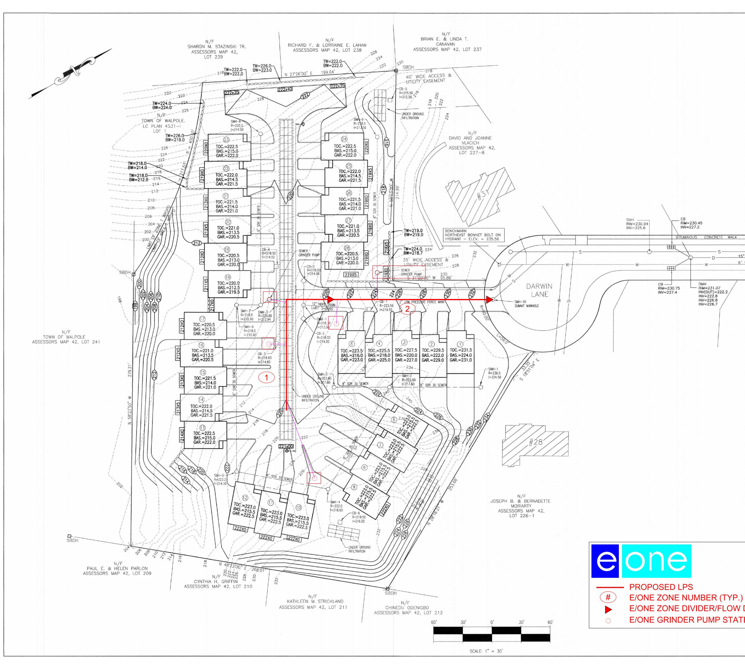
E/ONE ZONE DIVIDER/FLOW DIRECTION (TYP.) E/ONE GRINDER PUMP STATION (TYP.)
