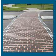
Description: Special paving treatments for crosswalks, which can include brick/pavers, colored or stamped asphalt, or thermoplastic pavement markings. Decorative crosswalks can be designed to reflect the unique character or identity of an area or neighborhood.
