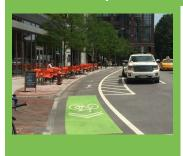
**Description:** A bicycle lane with additional striped space or textured pavement to increase the distance between the bicycle lane and adjacent traffic. Vertical elements that do not represent a permanent physical barrier (i.e. flex posts or tubular markers) may be used to provide physical separation from travel lanes.
