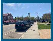
**Description:** Provision of on-street parking on one or both sides that reduces roadway width. Parked vehicles also provide a buffer between traffic and pedestrians on the sidewalk.
