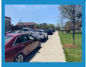
**Description:** Walkway parallel to the road that is intended for use by pedestrians, often with numerous access points to adjacent land uses. The pathway is typically physically separated from the roadway with a curb and/or verge.
