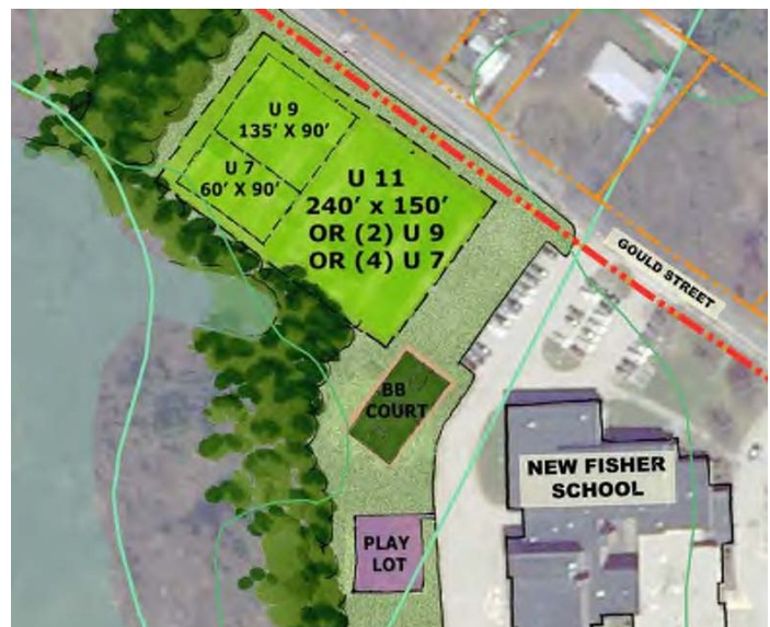
The recommended master plan showing the expanded U11 field and the relocated basketball court
