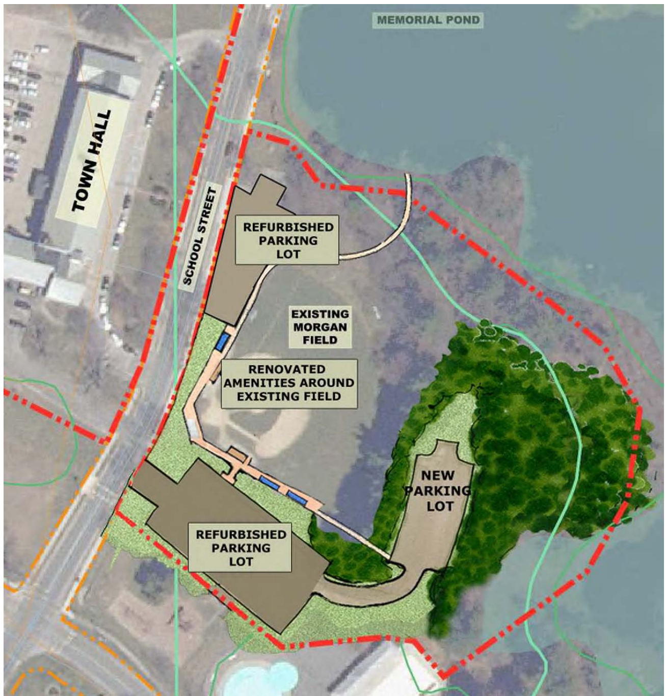
The preferred master plan for Morgan Field showing the reconfigured parking area, new gravel parking area to the back of the site and the increased green space between the parking lot and the field.
