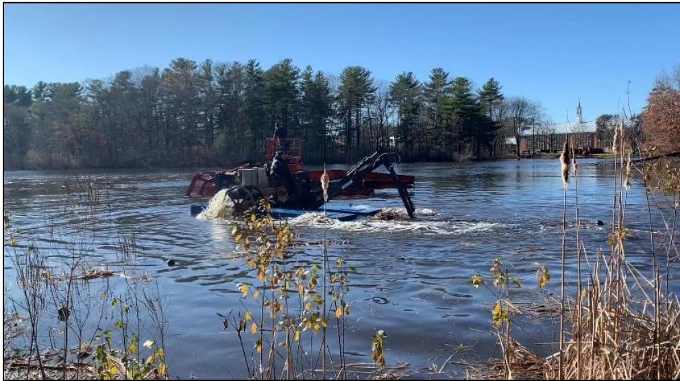
Hydroraking occurring at Memorial Pond – Fall 2019
